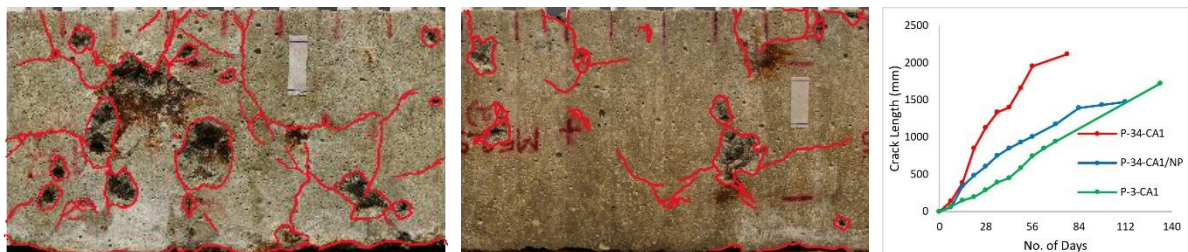
Figure 3.3: Pictures of P-34-CA1 (left) and P-34-CA1/NP (middle) specimens after 77 and 112 days of EAT exposure, respectively, and the corresponding crack length increment data (right)
