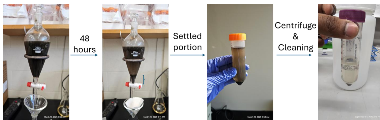
Figure 3: The flow of experiments utilized to concentrate the iron sulfides.
