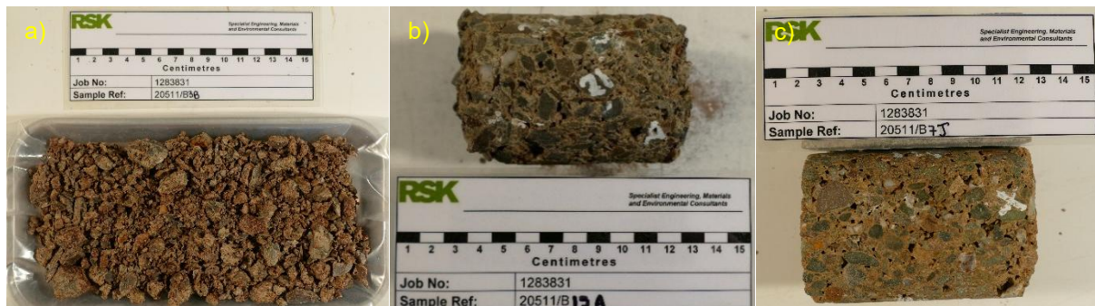
Figure 3.4 Photographs of the different failure morphologies a) complete failure, b) partial failure (heavily cracked, loss of stud(s)), c) Localised failure under measurement studs.
