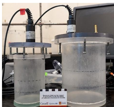
Figure 2.1: OCT cells used in the different trials of OCT interlaboratory studies; on the right-hand side, the original (larger) cell (OCT trial 1) and on the left-hand side, the new (smaller) cell (OCT trial 2). Testing parameters used for Trial 1 (with original cell) and Trial 2 (new (small) cell).
