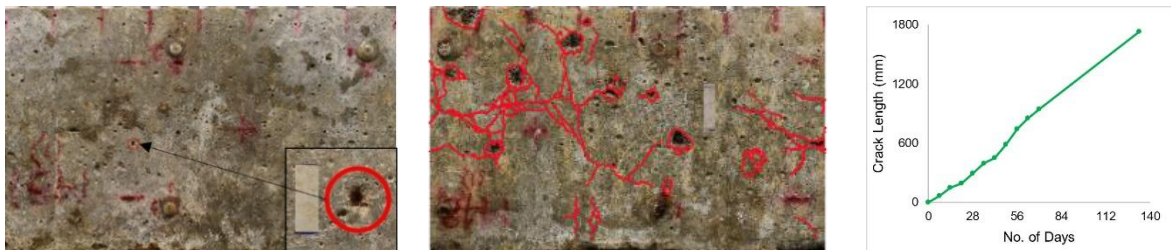
Figure 3.1: Pictures of P-1-CA1 (left) and P-3-CA1 (middle) specimens after 133 days of EAT exposure, and the corresponding crack length increment data for P-3-CA1 (right)
